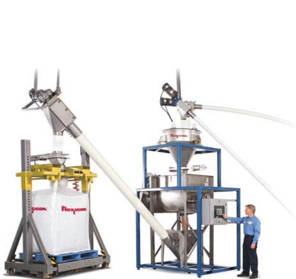
Flexicon's Self-Contained, Gain-in-Weight Batching and Blending System conveys bulk ingredients from multiple upstream sources, weigh-batches, blends and discharges the material into a surge hopper, and transports it to a TWIN-CENTERPOST™ Bulk Bag Filler. The system is offered with Flexicon Flexible Screw Conveyors (shown) or Flexicon Pneumatic Conveying Systems.
