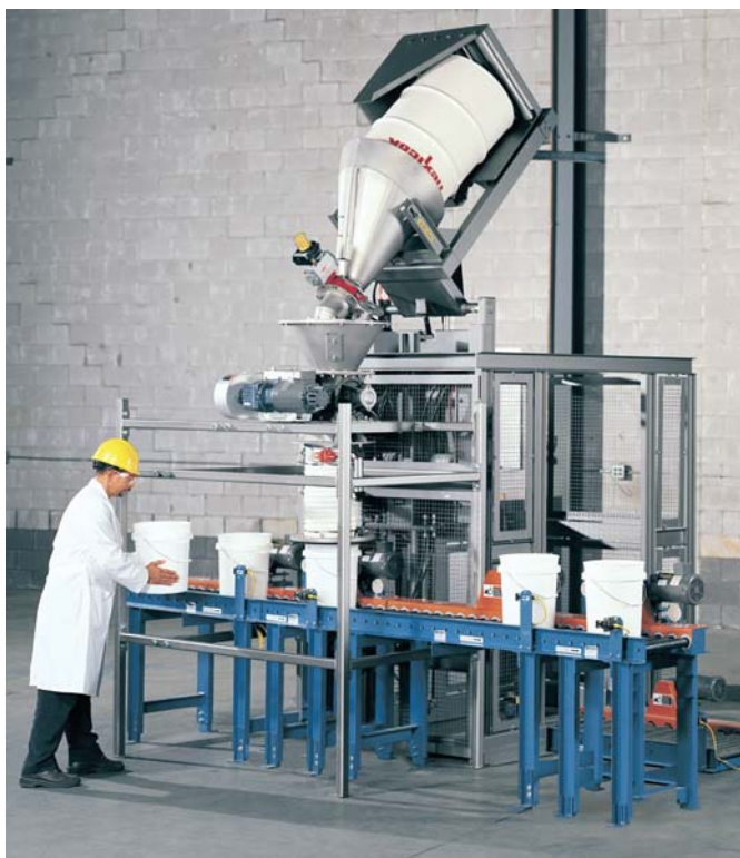
Flexicon's Bulk Filling System with High-Lift Drum Dumper allows drums to be loaded at floor level, sealed against a discharge cone, elevated and tipped, mating the cone spout to a receiver on the filling machine's surge hopper lid. The spout's slide gate valve opens to fill the hopper with no dusting, while pails are indexed, filled by weight, then conveyed to a second scale for check weighing.
