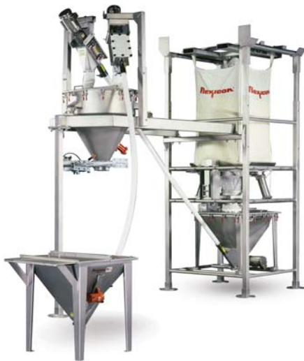
This Gain-in-Weight Batching System allows automated weighing of a major ingredient supplied in bulk bags, and a minor ingredient dumped manually. The central weigh hopper's load cells transmit weight gain information to a controller that starts and stops the conveyors to weigh each material in sequence, and actuates a slide gate valve to discharge the weighed batch.
