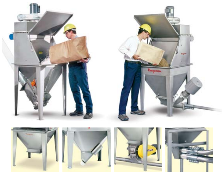
The hoppers of Flexicon Bag Dump Stations are offered with outlets configured for: (left to right) direct connection to process equipment, flexible screw conveyor charging adapters, rotary airlock valves with flow-through adapters, and non-flow-through pick-up adapters for multiple conveying lines.
