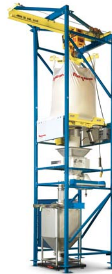
Flexicon's Bulk-Bag-to-Rigid-Tote Weigh Batching System seals against the clean side of the bag spout, elongates the bag for total evacuation, and allows dust-free retying of partially empty bags. A low-profile de-lumping device breaks up agglomerates as a gravimetric feeder loads accurately weighed batches into rigid totes.
